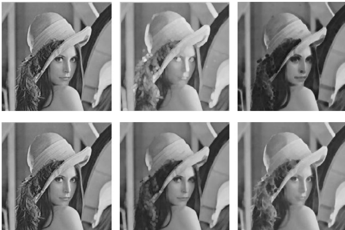
Figure 2.3: Results examples of grayscale dilation (Top Middle), erosion (Top Right), opening (Bottom Middle), closing (Bottom Right). Original image on the left (Top and Bottom). Images from Yu (2004)
